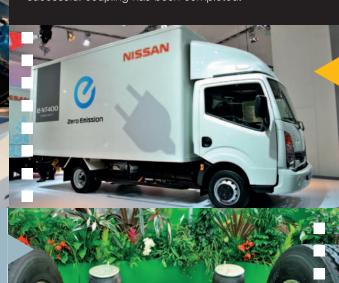
van, Nissan displayed another electric vehicle in its range, albeit in concept form. The Cabster refrigerated van uses a diesel engine, in combination with a 48kw/h battery pack - comprising two of the packs found in the Nissan LEAF car. The vehicle offers a range of 140km, making it ideal for operators involved in city distribution. Nissan also confirmed that, while the Cabster is likely to make it to production, the plan is not to electrify every vehicle in the range.
