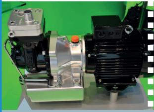
Catering to the bus and hybrid heavy duty truck markets, Wabco showcased its new, electrically-driven air compressor, dubbed e-comp. Claiming to help improve fuel efficiency by up to 35%, its 6kW motor is currently undergoing testing on hundreds of prototypes around the world, according to the company. Most of these vehicles can be found in China, but Europe is also trialling the technology, with positive feedback so far.
